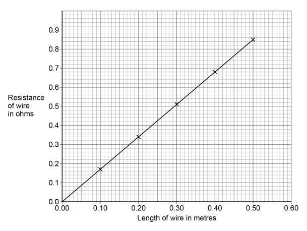
Describe the relationship between the length of the wire and the resistance of the wire.
